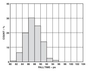
Figure 5. Fall Time Distribution Under Worst-Case Operating Conditions
