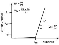
Figure 6. Laser Transfer Function
