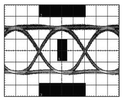
Figure 14. A 2.5 Gbps Optical Eye at 85°C. Average Power = 0 dBm, Extinction Ratio = 10 dB, PRBS 31 Pattern. Eye Obtained Using a DFB Laser.
