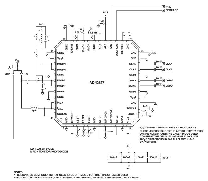
Figure 12. AC-Coupled 50 Mbps to 3.3 Gbps Test Circuit, Data Not Clocked
