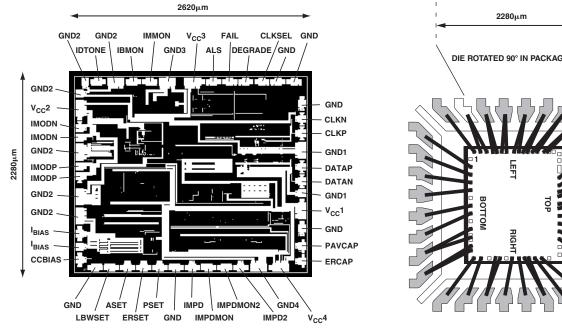
Figure 2. Metallization Photograph
