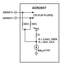
Figure 7. AC Coupling of Data Inputs
