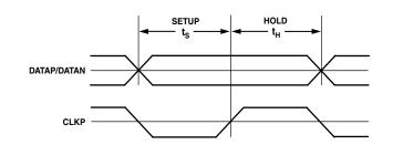
Figure 1. Setup and Hold Time
