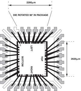
Figure 3. Bonding Diagram
