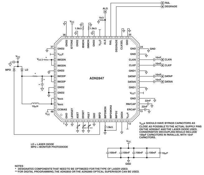
Figure 11. DC-Coupled 3.3 Gbps Test Circuit, Data Not Clocked
