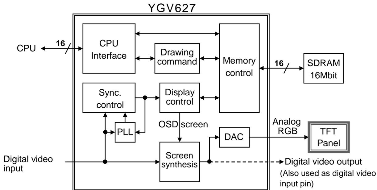
YGV627 is connected to the external memory bus of CPU as an external I/O device. As a video memory, SDRAM of up to 64M bits can be connected to local memory bus of YGV627 to send bitmap image data stored in the video memory into monitor as RGB signal in accordance with display scan timing.
