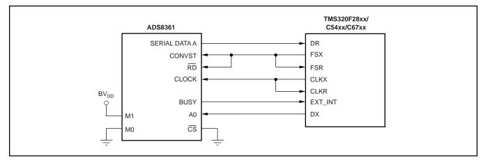
FIGURE 15. 2x2 Channel Using A Output.
