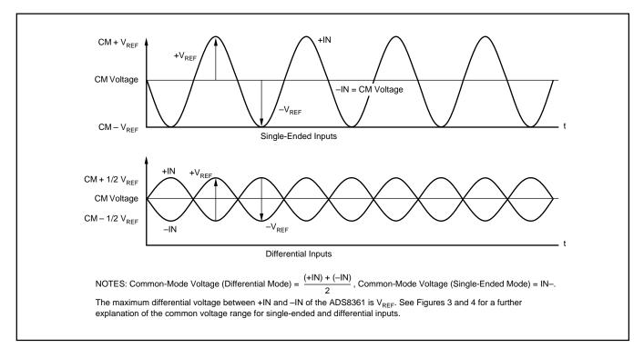
FIGURE 2. Using the ADS8361 in the Single-Ended and Differential Input Modes.
