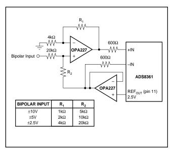
FIGURE 7. Level Shift Circuit for Bipolar Input Ranges.
