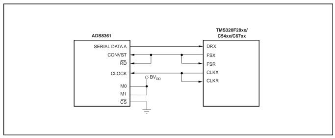
FIGURE 17. 4-Channel Sequential Mode Using A Output.
