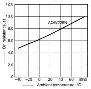
2.-(2) On resistance vs. ambient temperature characteristics
