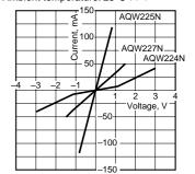
9. Off state leakage current
