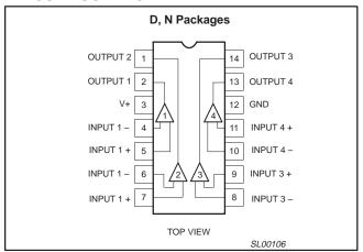
Figure 1. Pin Configuration
