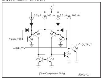
Figure 2. Equivalent Circuit
