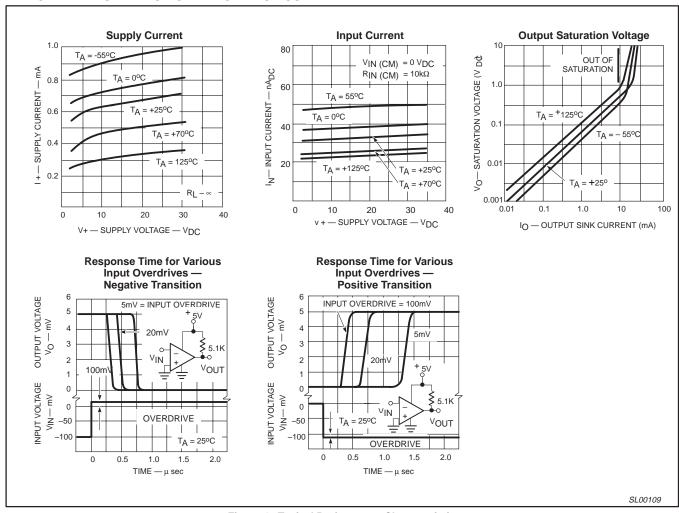
Figure 4. Typical Performance Characteristics
