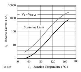
Figure 1. Reverse Current vs. Junction Temperature
