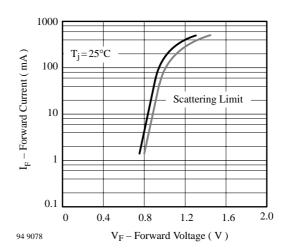
Figure 2. Forward Current vs. Forward Voltage
