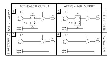
Table 1. PEEL<sup>TM</sup>22CV10A Macrocell Configuration Bits
