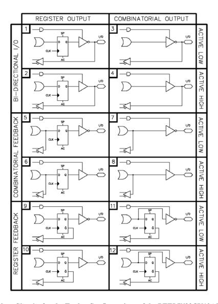
Figure 22 Equivalent Circuits for the Twelve Configurations of the PEEL<sup>TM</sup>22CV10AZ+ I/O Macrocell
