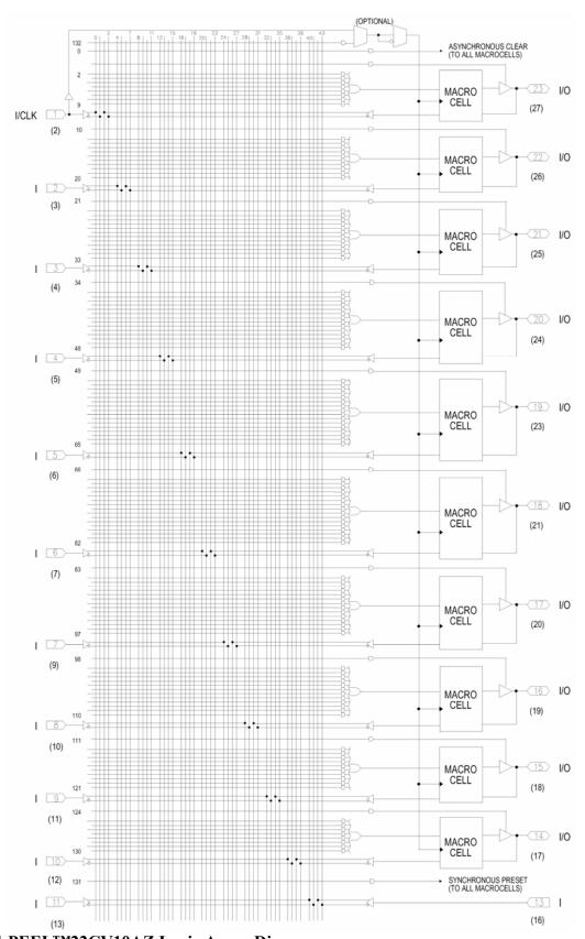
Figure 21 PEELTM22CV10AZ Logic Array Diagram
