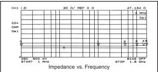
Impedance is measured using an HP4291A S-Parameters are measured using an HP8753C
