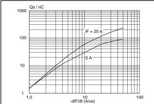
Fig.8. Maximum  $Q_s$  at  $T_i = 25$ °C; per diode
