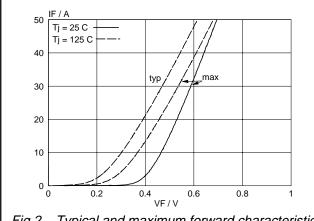
Fig.2. Typical and maximum forward characteristic  $I_F = f(V_F)$ ; parameter  $T_i$
