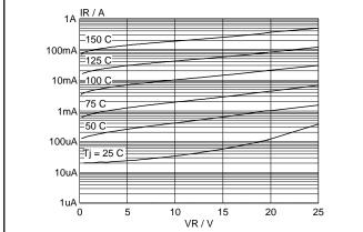
Fig.3. Typical reverse leakage current per diode;  $I_R = f(V_R)$ ; parameter  $T_j$
