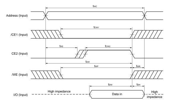
Cautions 1. During address transition, at least one of pins /CE1, CE2, /WE should be inactivated.
