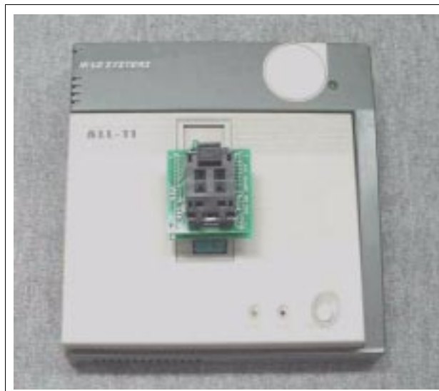
Figure 9-2 ALL-11 Programmer with adapter
