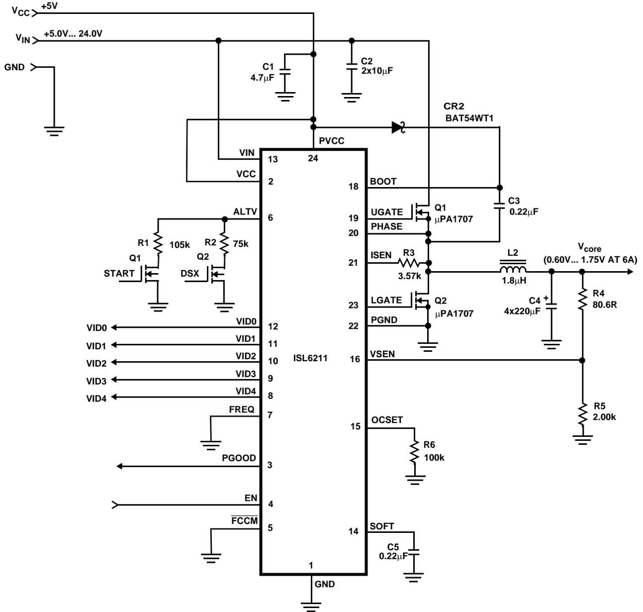
FIGURE 13. APPLICATION CIRCUIT
