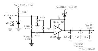
FIGURE 4a. Low Drift Extremely Stable Reference Circuit
