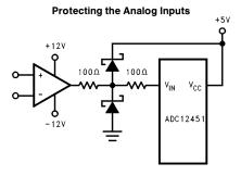
Note: External protection diodes should be able to withstand the op amp current limit.
