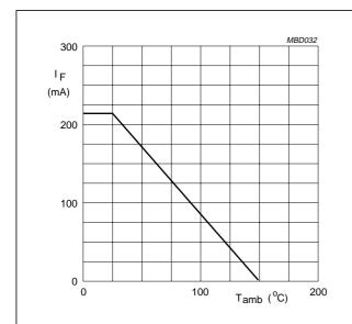
Device mounted on an FR4 printed-circuit board.
