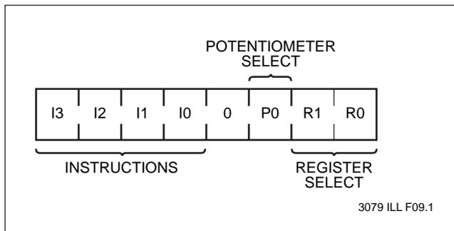
The four high order bits define the instruction. The sixth bit (P0) selects which one of the two potentiometers is to be affected by the instruction. The last two bits (R1 and R0) select one of the four registers that is to be acted upon when a register oriented instruction is issued.
