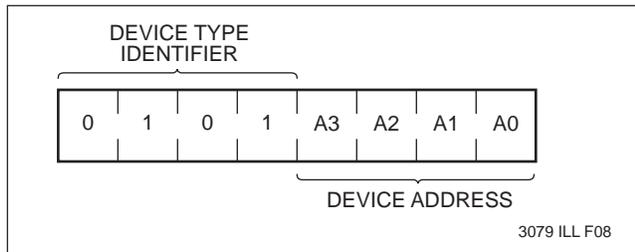
The next four bits of the slave address are the device address. The physical device address is defined by the state of the A0-A3 inputs. The X9221 compares the serial data stream with the address input state; a successful compare of all four address bits is required for the X9221 to respond with an acknowledge.
