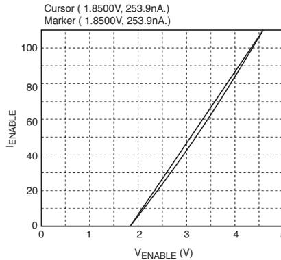
12mA ENABLE Current vs. ENABLE Voltage
