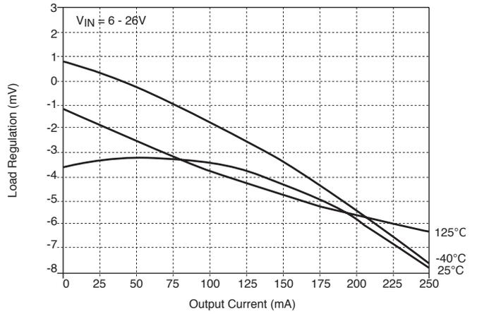
Load Regulation vs Output Current for  $V_{OUT2}$
