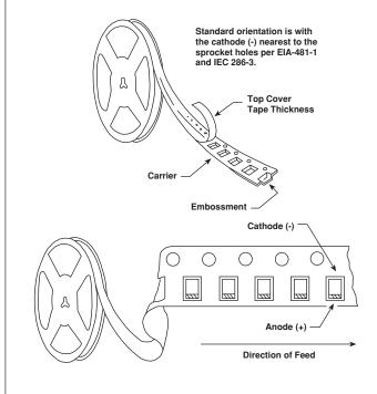
**Tape and Reel Specifications**: All case codes are available on plastic embossed tape per EIA-481-1. Tape reeling per IEC 286-3 is also available. Standard reel diameter is 7" [178mm]. 13" [330mm] reels are available.
