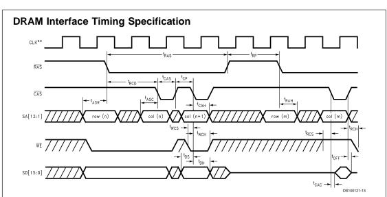
\*\*The CLK signal is only included as a reference; no specifications are guarantee to this signal. FIGURE 8. DRAM Timing Diagram
