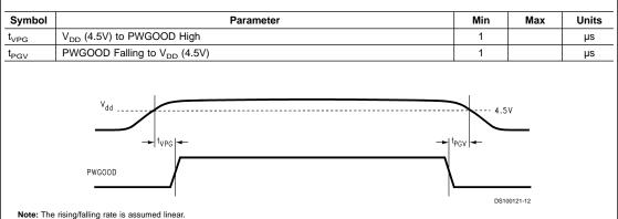
FIGURE 7. PWGOOD in Relation to V<sub>DD</sub>
