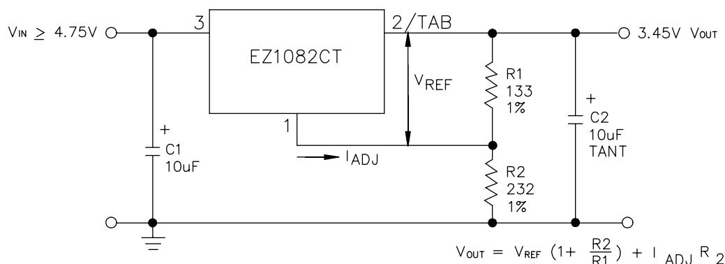
(1) C1 NEEDED IF DEVICE IS FAR FROM FILTER CAPACITORS.
