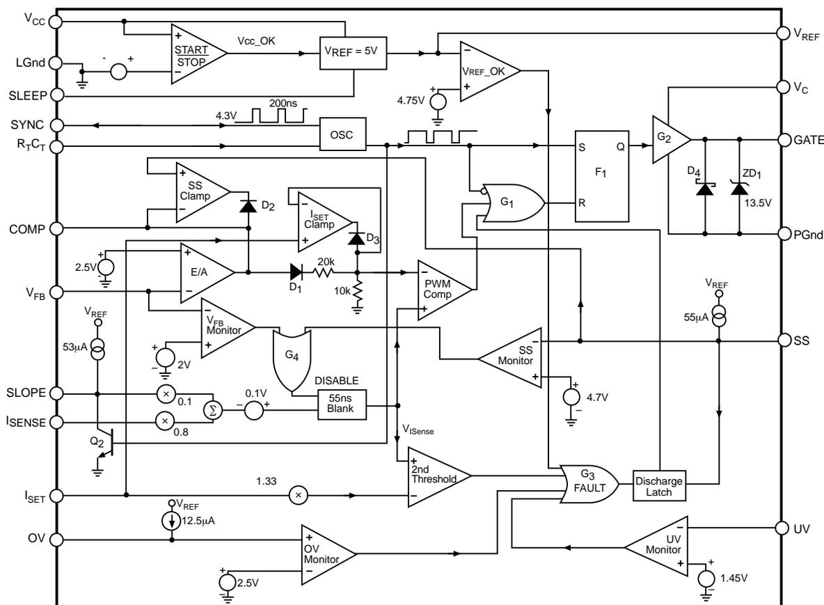
Figure 1: CS51021/22/23/24 Block Diagram
