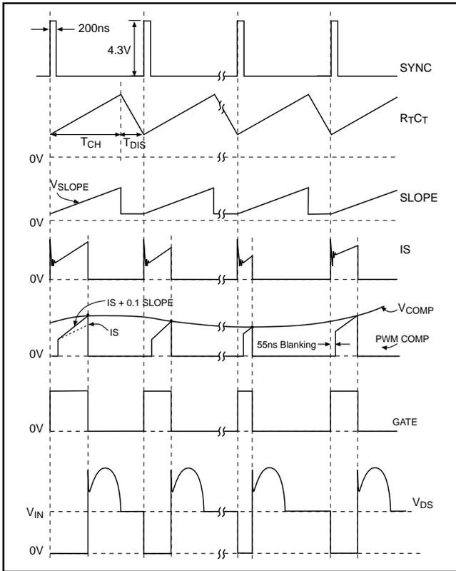
Figure 2: Typical Waveforms
