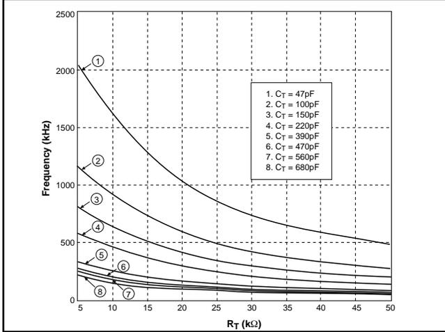
Figure 5: Frequency vs.  $R_T$  for Discrete Capacitor Values.
