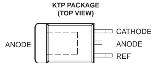
The ANODE terminal is in electrical contact with the mounting base.
