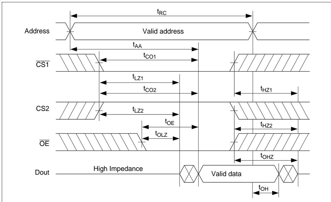
Read Timing Waveform (2) ( $\overline{WE} = V_{IH}, \overline{OE} = V_{IL}$ )
