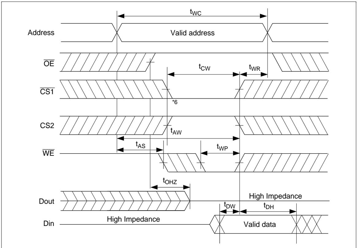
Write Timing Waveform (2) ( $\overline{OE}$  Low Fixed) ( $\overline{OE} = V_{IL}$ )
