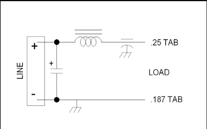
The ZA -1193-3C is an interference filter specifically designed for use in the automotive environment.
