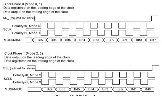
Figure 15: SPI Waveforms
