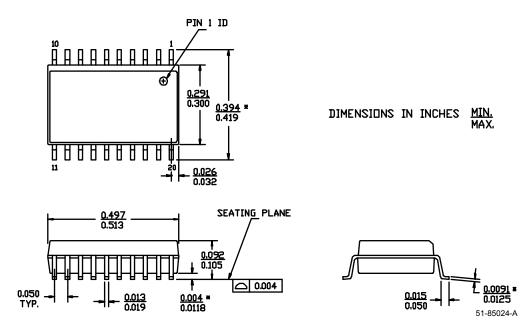
Figure 43: 20-Lead (300-Mil) Molded SOIC S5
