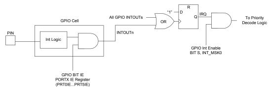
Figure 11: GPIO Interrupt Enable Diagram
