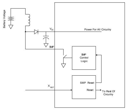
Figure 32: Switch Mode Pump
