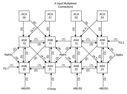
**Figure 22: AMux Connections**
