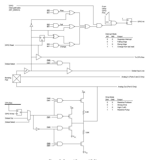
Figure 7: General Purpose I/O Pins
