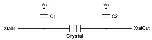
Figure 8: External Crystal Oscillator Connections
