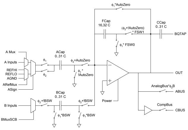
Figure 25: Analog Switch Cap Type B PSoC Blocks
