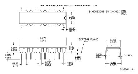
Figure 40: 20-Lead (300-Mil) Molded DIP P5
