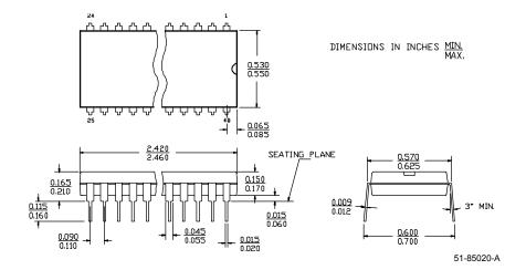
Figure 42: 48-Lead (600-Mil) Molded DIP P25
