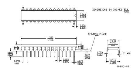
Figure 41: 28-Lead (300-Mil) Molded DIP P21
