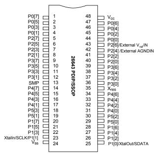
Figure 6: 26643 PDIP/SSOP
