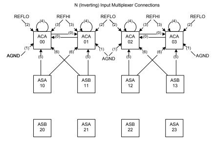
**Figure 17: NMux Connections**
