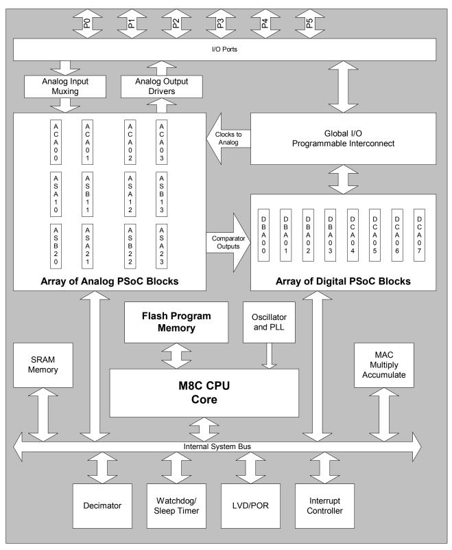
Figure 1: Block Diagram
