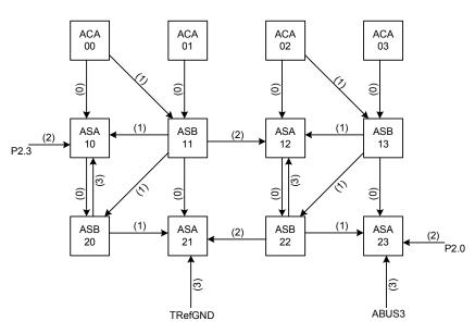
Figure 24: BMuxSCA/SCB Connections
