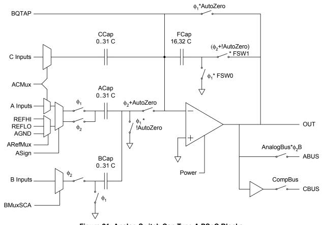
Figure 21: Analog Switch Cap Type A PSoC Blocks
