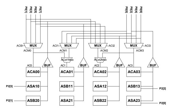
Figure 26: Analog Input Muxing
