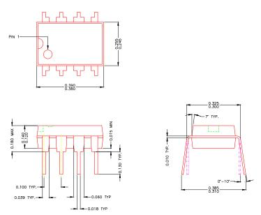
Figure 45: 8-Lead (300-Mil) Molded DIP
