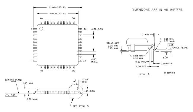
Figure 36: 44-Lead Thin Plastic Quad Flat Pack A44
