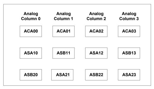
Figure 16: Array of Analog PSoC Blocks
