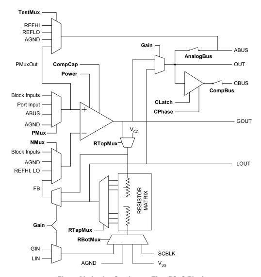
Figure 20: Analog Continuous Time PSoC Blocks
