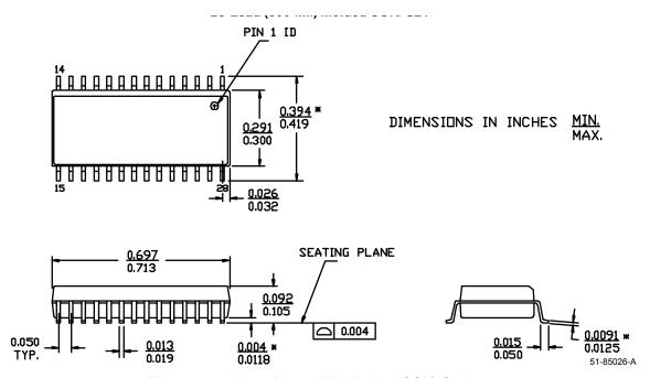
Figure 44: 28-Lead (300-Mil) Molded SOIC S21
