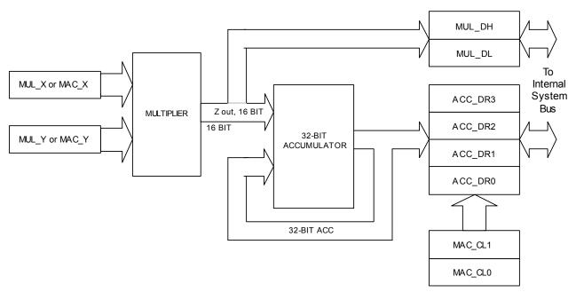
Figure 28: Multiply/Accumulate Block Diagram
