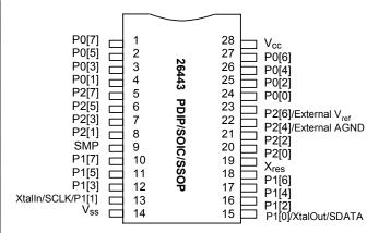
Figure 4: 26443 PDIP/SOIC/SSOP
