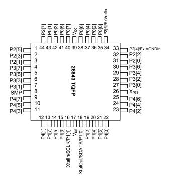
Figure 5: 26643 TQFP
