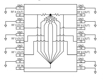
PINS 1,3,5,7,9,12,14,16,18 AND 20 SHOULD BE DC AND RF GROUNDED.
