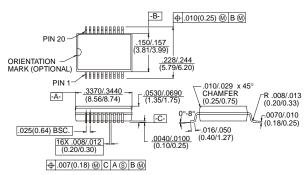
20-Lead SSOP outline dimensions (All dimensions per JEDEC No. MS-137-AD, Issue C)
