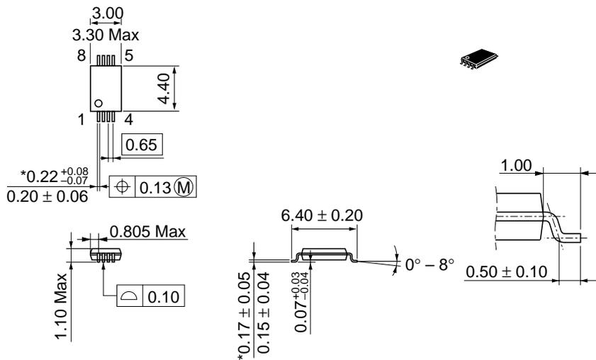
\*Dimension including the plating thickness
