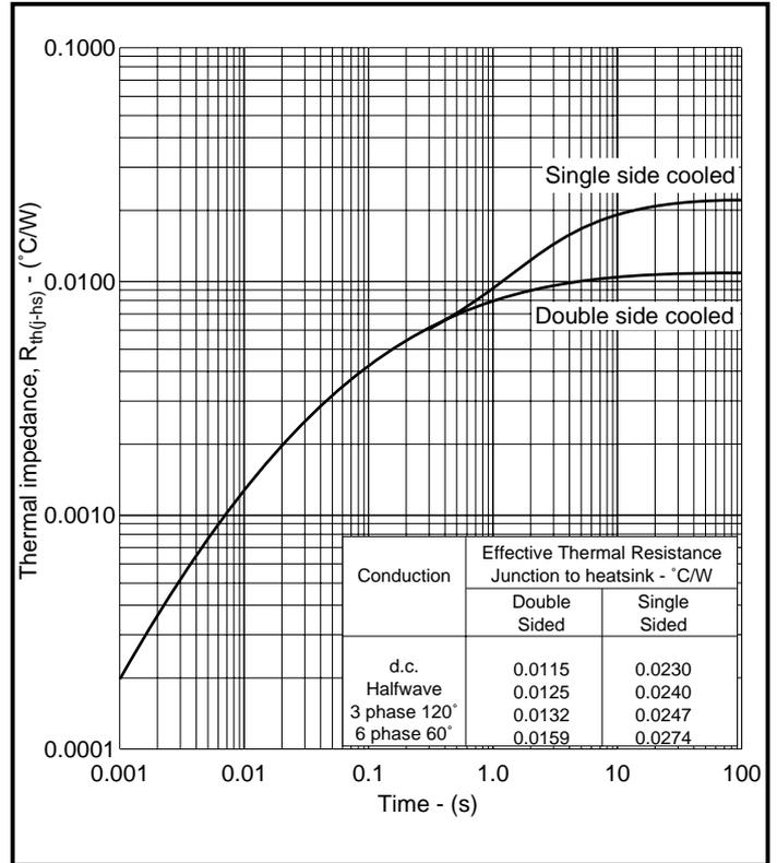
Fig.6 Transient thermal impedance - junction to heatsink
