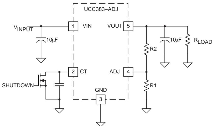
Figure 5. Typical Application for 5-Pin Adjustable Version
