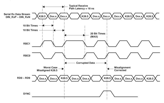
Figure 2. Word Realignment Timing Characteristics Waveforms
