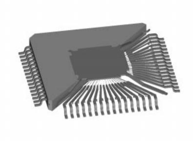
Figure 9. Heat-Spreader Design
