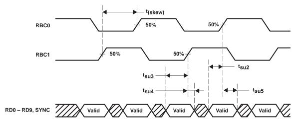
Figure 7. Receiver Interface Timing Waveforms
