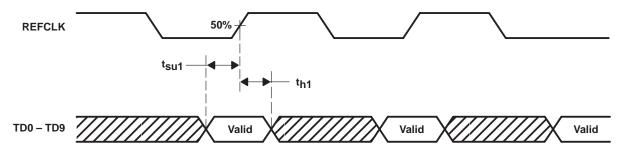
Figure 4. Transmit 10-Bit Interface Timing Waveforms
