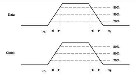
Figure 6. Receiver Data Measurement Levels
