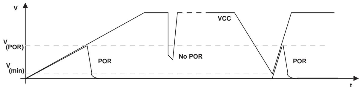
Figure 3. Power-On Reset (POR) vs Supply Voltage
