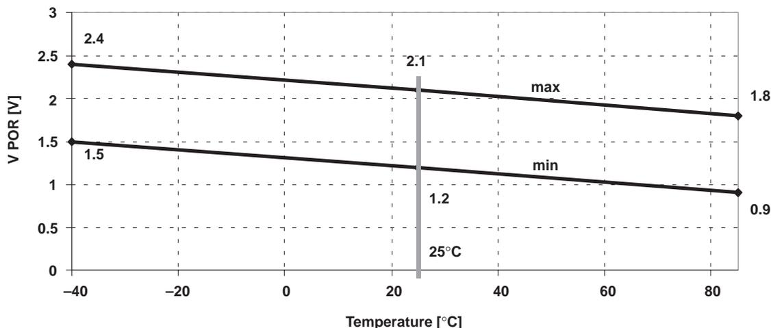
Figure 4. V<sub>(POR)</sub> vs Temperature
