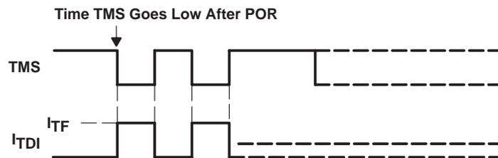
Figure 6. Fuse Check Mode Current, MSP430C33xA
