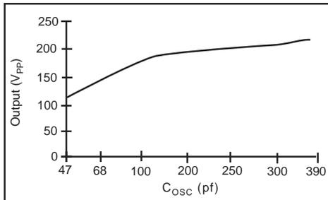
Output Voltage vs. C<sub>osc</sub>
