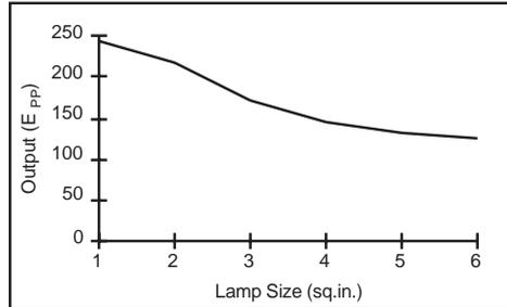
Output Voltage vs Lamp Size.
