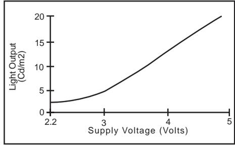
Luminance vs. V<sub>DD</sub>=V<sub>coil</sub>
