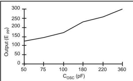
Output Voltage vs C<sub>osc</sub>
