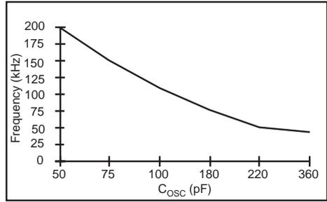
Oscillator Frequency vs C<sub>osc</sub>
