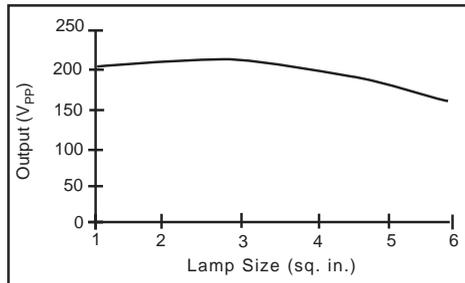
Output Voltage vs. Lamp Size.
