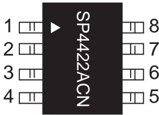
Pin 1 – HON- Enable for driver operation, high = active; low = inactive.
