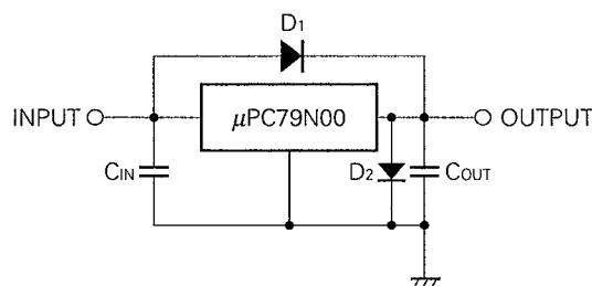
$C_{IN}$ : More than 2.2  $\mu\text{F}$ . $C_{OUT}$ : More than 1  $\mu\text{F}$ .D1: Needed for  $V_{IN} > V_o$ .D2: Needed for  $V_o > \text{GND}$ .
