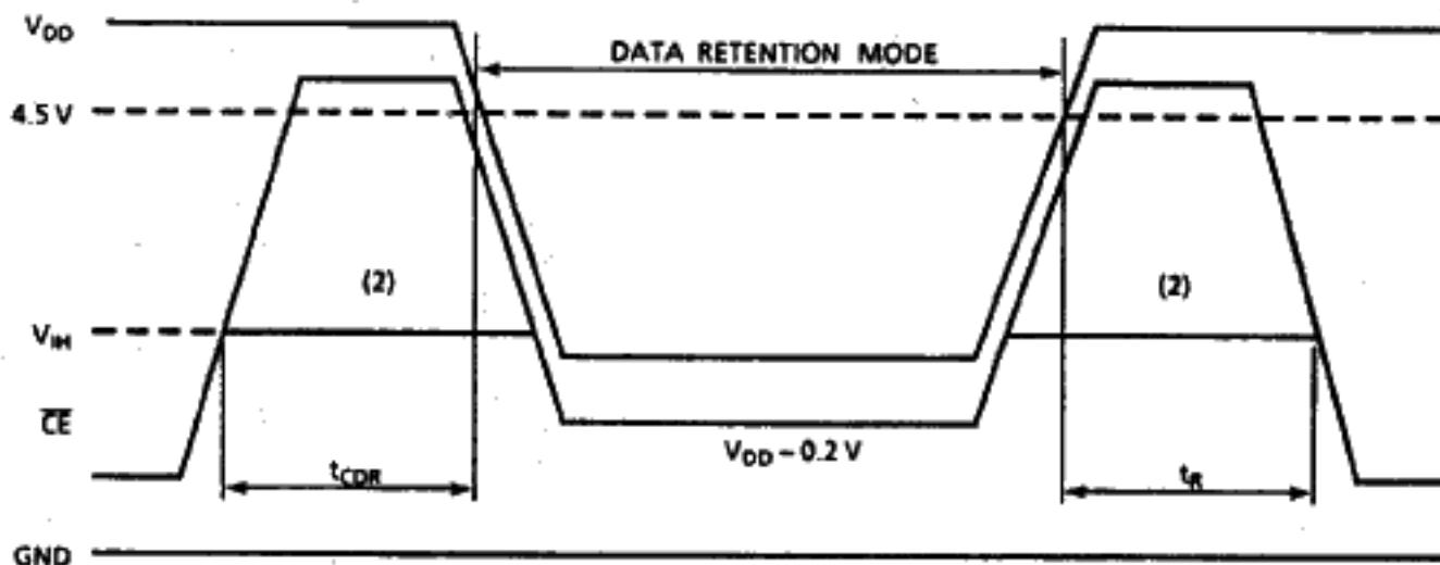
Note (2): If the  $V_{IH}$  of  $\overline{CE}$  is 2.4V in operation,  $I_{DD2}$  current flows during the period that the  $V_{DD}$  voltage is going down from 4.5V to 2.6V.
