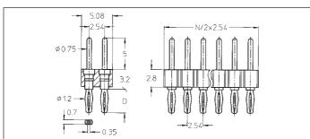
for PCB thickness 1.5 to 2.0 mm D = 2.80 mm 802-10-xxx-65-001 802-90-xxx-65-001
