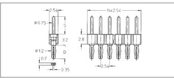
for PCB thickness 1.5 to 2.0 mm D = 2.80 mm 800-10-xxx-65-001 800-90-xxx-65-001
