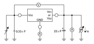
FOR RIPPLE REJECTION RATIO
