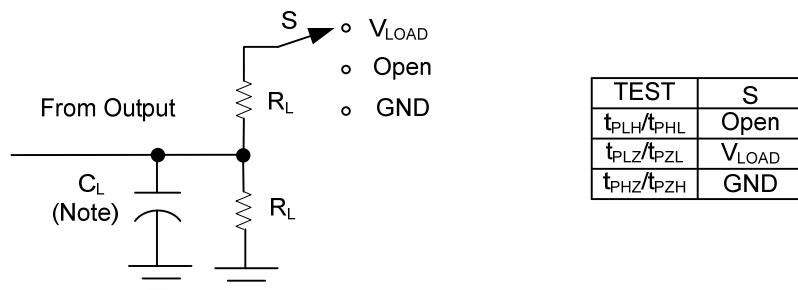
Note:  $C_L$  includes probe and jig capacitance.
