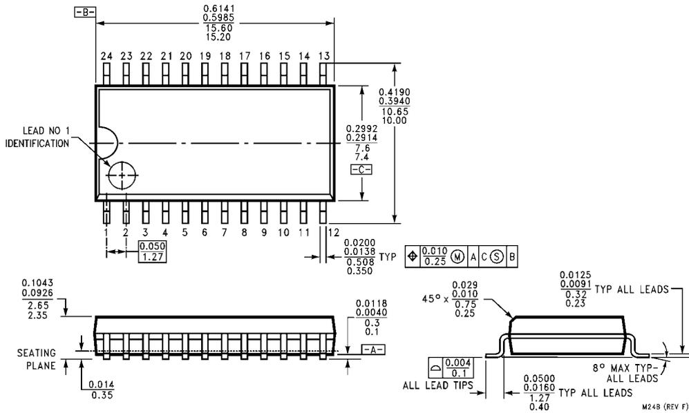
**28-Lead Small Outline Integrated Circuit (SOIC), JEDEC MS-013, 0.300 Wide
