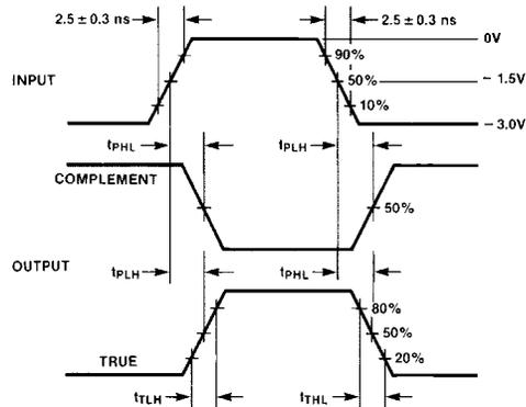
FIGURE 1. Propagation Delay, Cut-Off and Transition Times
