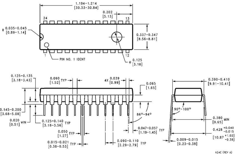
**24-Lead Plastic Dual-In-Line Package (PDIP), JEDEC MS-010, 0.400 Wide
