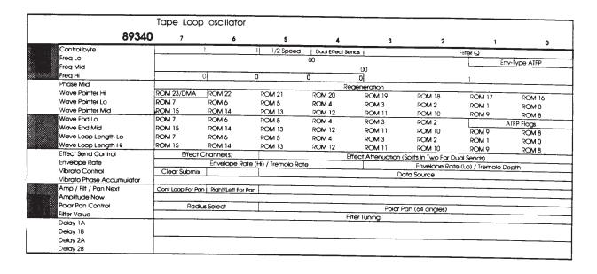
Figure 12. The Tape Loop Oscillator Address Map
