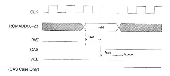
Figure 5. Sample Memory Address Timing Diagram
