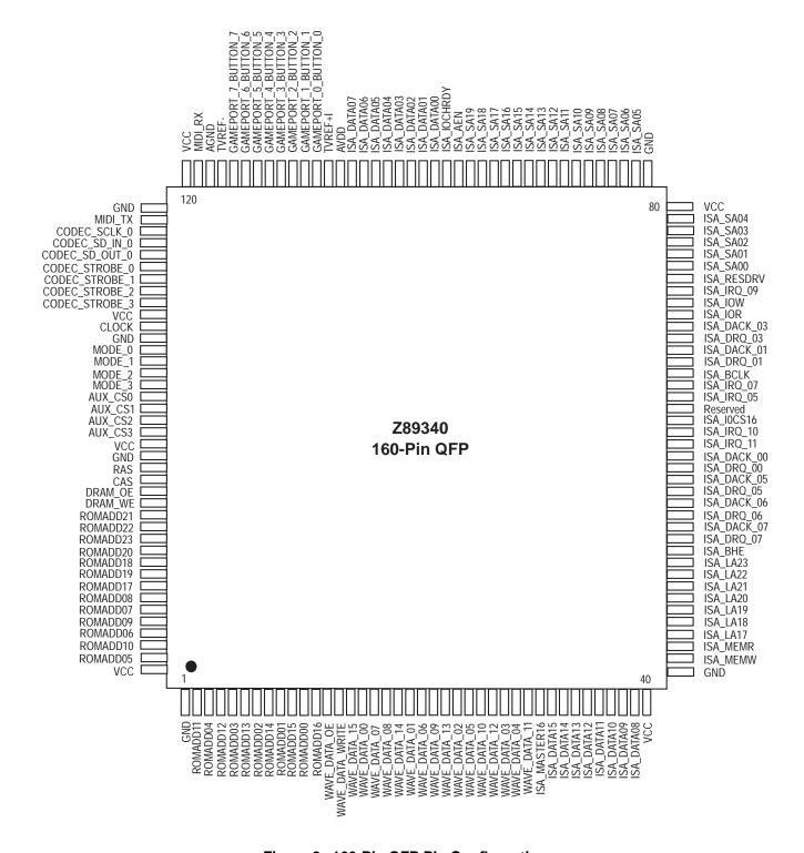
Figure 2. 160-Pin QFP Pin Configuration
