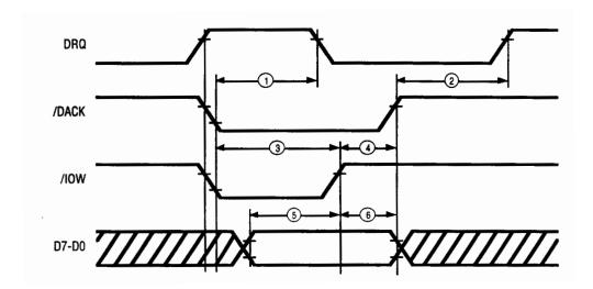
Figure 3. DMA Write Timing Diagram
