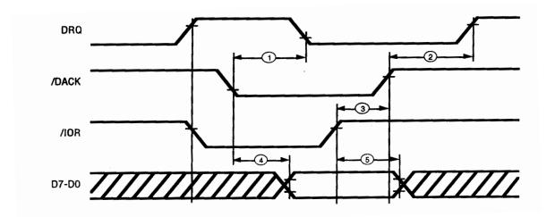
Figure 4. DMA Read Timing Diagram
