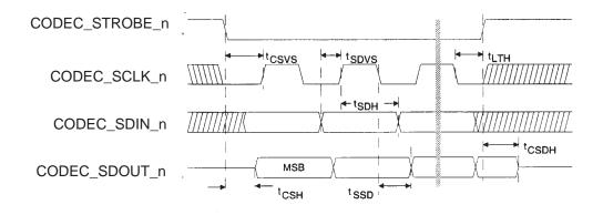
Figure 9. CODEC Interface Timing Diagram
