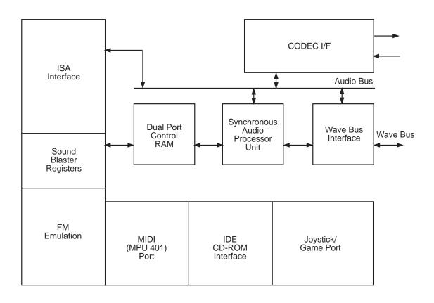
Figure 1. Z89340 Simplified Functional Block Diagram
