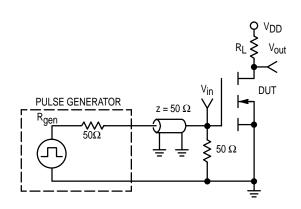
Figure 10. Switching Test Circuit
