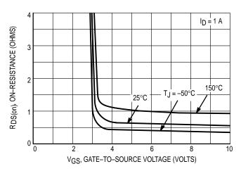
Figure 4. R<sub>DS(on)</sub> Variation With Gate-To-Source Voltage
