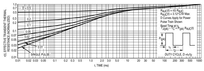
Figure 9. Thermal Response (MLP1N06CL)
