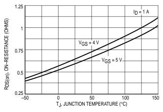
Figure 5. On–Resistance Variation With Temperature
