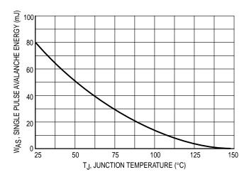
Figure 6. Single Pulse Avalanche Energy versus Junction Temperature
