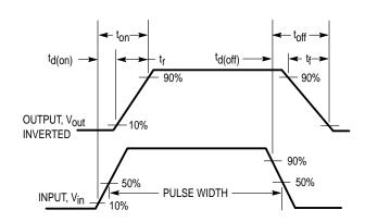
Figure 11. Switching Waveforms
