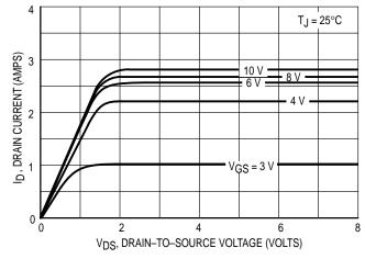
Figure 1. Output Characteristics
