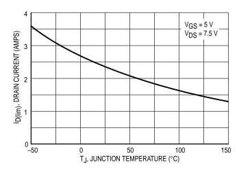
Figure 3. ID(lim) Variation With Temperature
