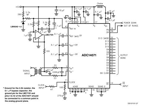
FIGURE 7. Driving the Signal Inputs with a Transformer
