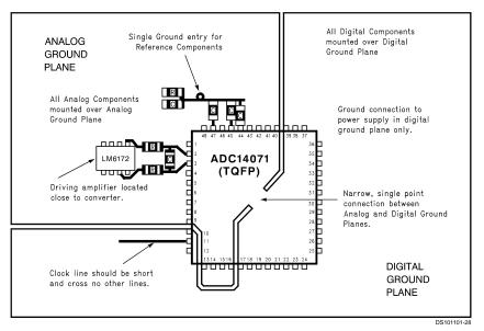
FIGURE 8. Example of A Suitable Layout
