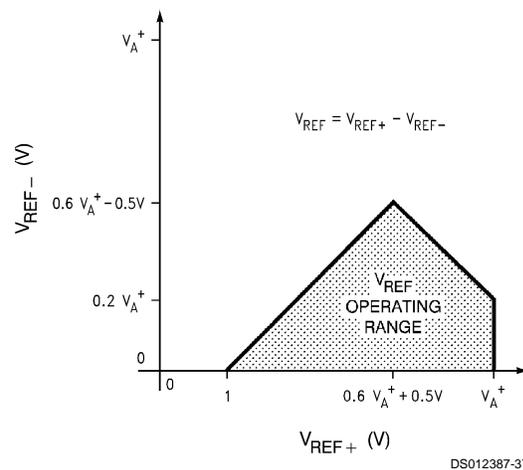
FIGURE 19.  $V_{\text{REF}}$  Operating Range
