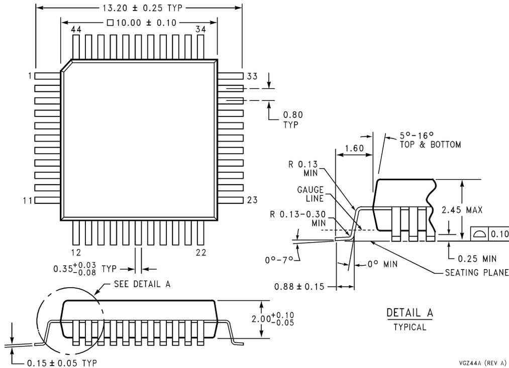
**44-Lead (10mm x 10mm) Molded Plastic Quad Flat Package**
