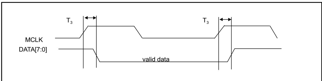
$T_3$  : MCLK rising to DATA valid maximum time : 18ns [output load: 60pF]
