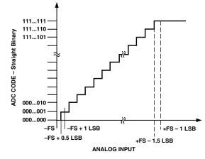
Figure 3. ADC Ideal Transfer Function
