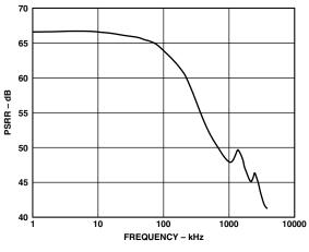
Figure 6. PSRR vs. Frequency
