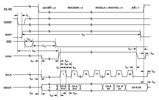
Figure 15. Master Serial Data Timing for Reading (Read after Convert)
