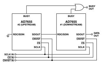
Figure 19. Two AD7655s in a Daisy-Chain Configuration
