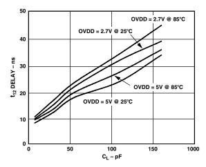
TPC 11. Typical Delay vs. Load Capacitance C<sub>L</sub>
