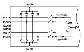
Figure 5. Simplified Analog Input
