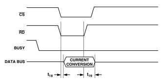
Figure 11. Slave Parallel Data Timing for Reading (Read after Convert)
