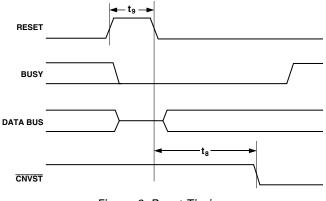
Figure 9. Reset Timing
