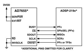
Figure 20. Interfacing the AD7655 to SPI Interface
