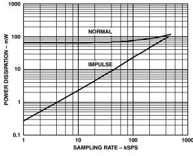
Figure 7. Power Dissipation vs. Sample Rate
