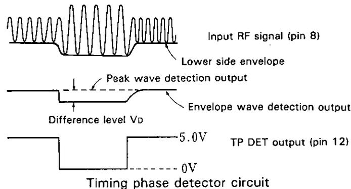
Timing phase detector circuit
