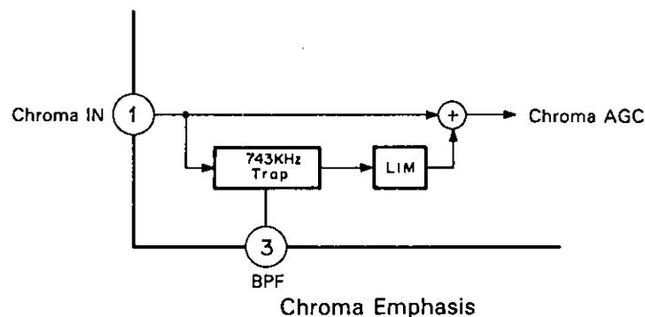
The down converted chroma signal is applied to the chroma Emphasis input, and the amount of emphasis diminishes around  $f_{sc}$  (color sub carrier frequency:  $743.444 \text{ kHz}$ ) as it is distanced from  $f_{sc}$ , the amount of emphasis grows.
