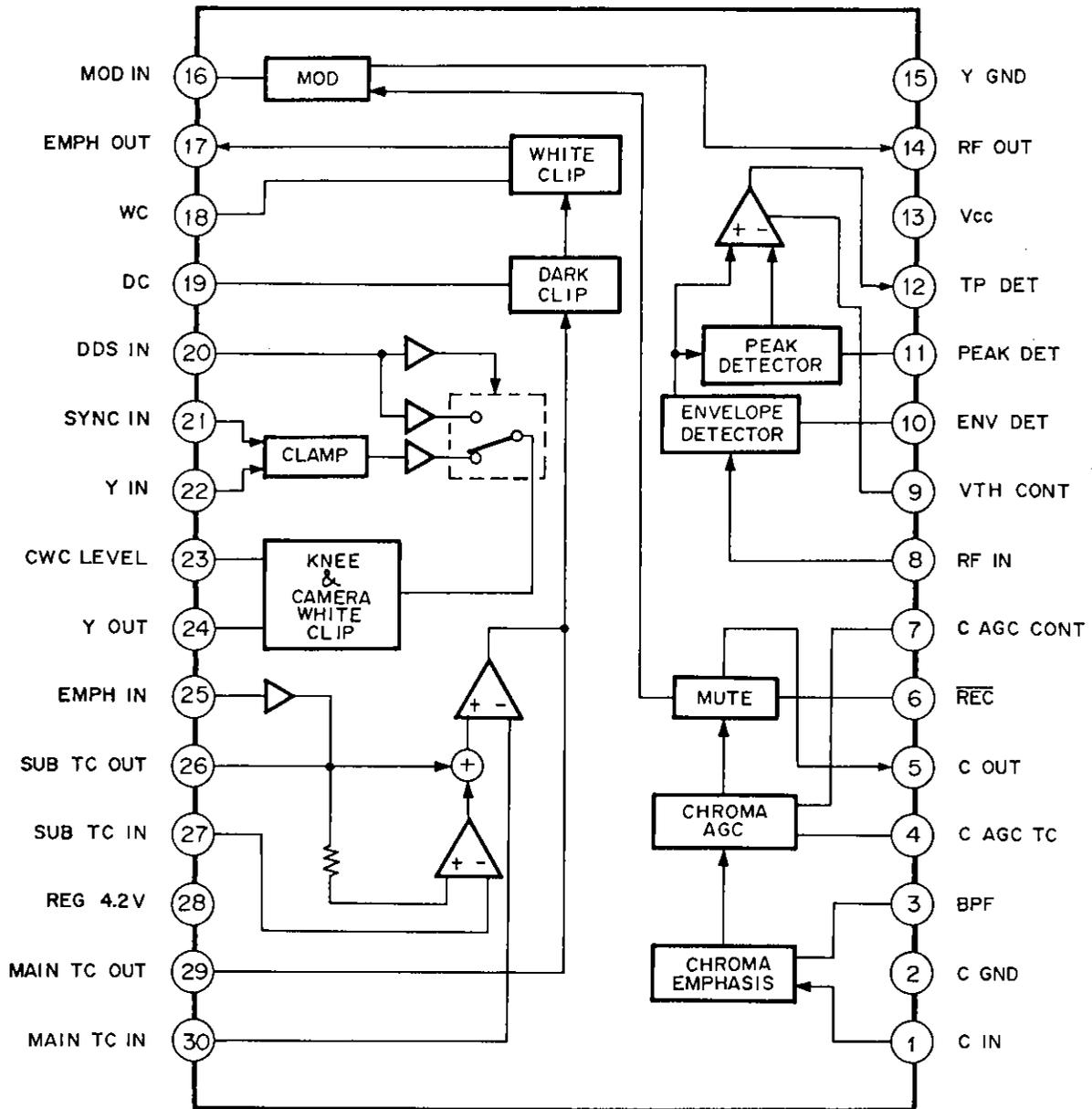
Pin Description and Equivalent Circuit
