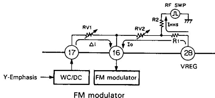
At the figure, (FM modulator) the carrier bias current  $I_0$  can be adjusted through  $RV_2$ . Also, the level (deviation) of signal current  $\Delta I$  can be set with  $RV_1$ . The HHS current ( $I_{HHS}$ ) is determined through  $R_1$ ,  $R_2$ , and RF SWP level.
