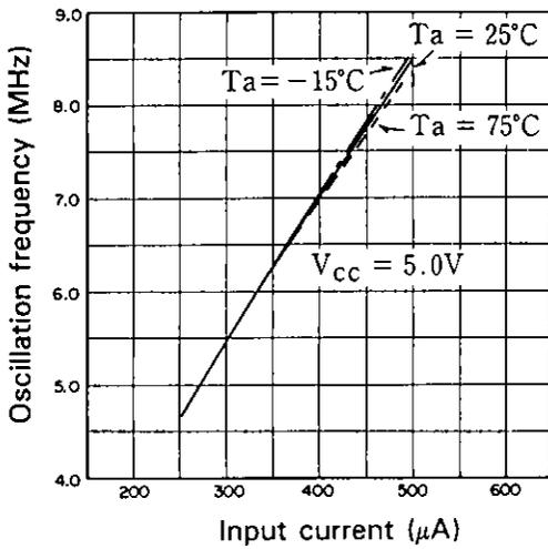
**FM MOD Oscillation frequency supply voltage characteristics**
