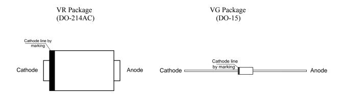
Figure 2. Pin Configuration of MBR2150 (Top View)
