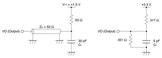
$\textbf{Remark} \;\; \textbf{CL} \; \text{includes capacitances of the probe and jig, and stray capacitances}.$
