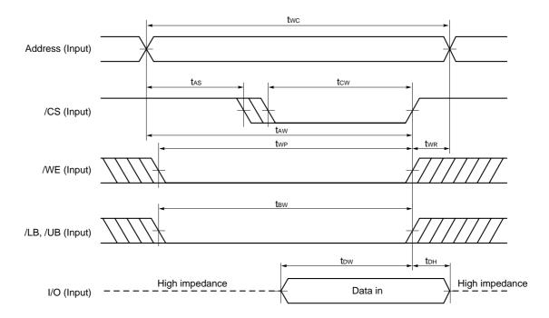
Cautions 1. /CS or /WE should be fixed to high level during address transition.
