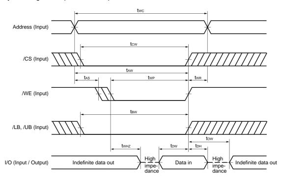
Cautions 1. /CS or /WE should be fixed to high level during address transition.
