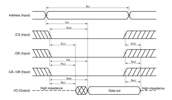
Caution Address valid prior to or coincident with /CS low level input.
