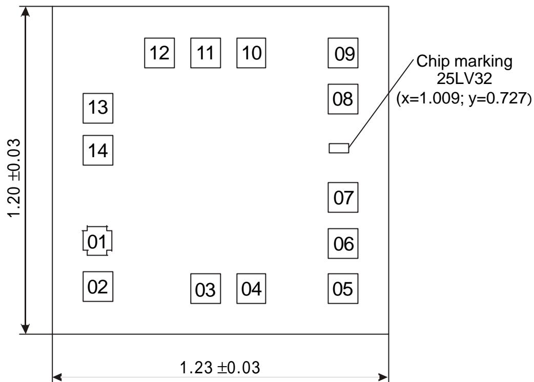
Pad size  $0.108 \times 0.108$  mm (Pad size is given as per metallization layer)
