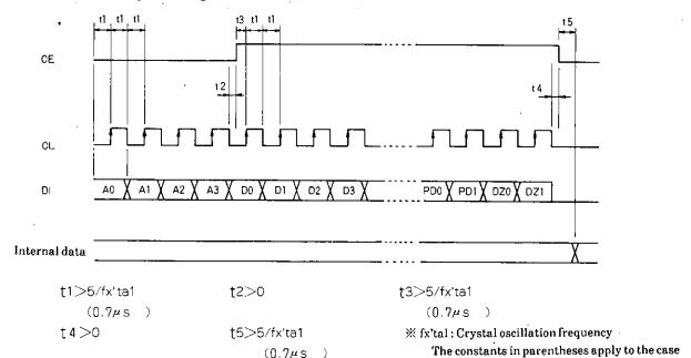
Mode 1: This mode allows the user to input 60 bits to the DI pin: 4 mode selection data bits + 56 control data bits
