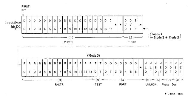
The sirial data for controlling the LM7005 consists of 56 bits. After the power on, all the 56 bits must be input to the LM7005 for initialization.
