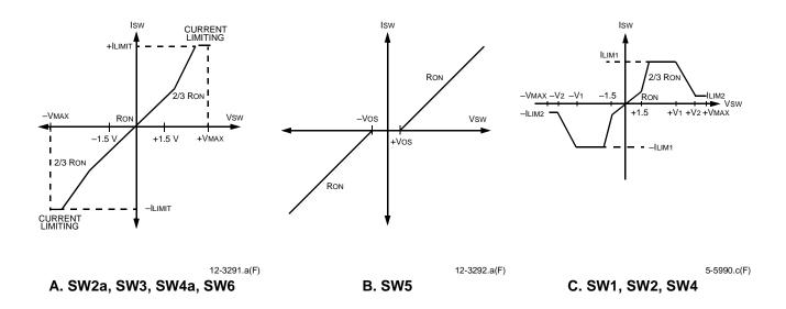
Figure 3. On-State Switch I-V Characteristics
